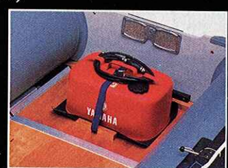
FUEL TANK PAD
