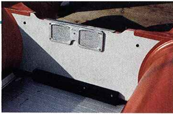
Fiberglass transoms with motor pads are featured on most Achilles sportboats.
