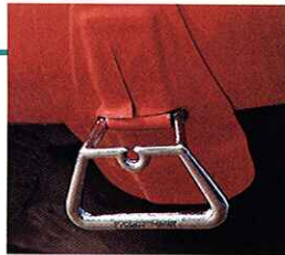
A heavy-duty stainless steel towing ring and bow camping handle are standard on Achilles sportboats and sport dinghies.
