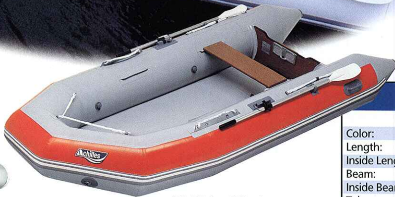
LSI-112 has 18" tubes and two rear carry handles.
