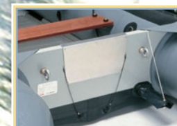
HEAVY-DUTY SELF-BAILER AND ALUMINUM-PLATED TRANSOM.
