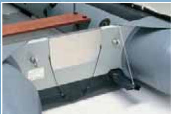
Heavy-duty Self-bailer and Aluminum-plated Transom
