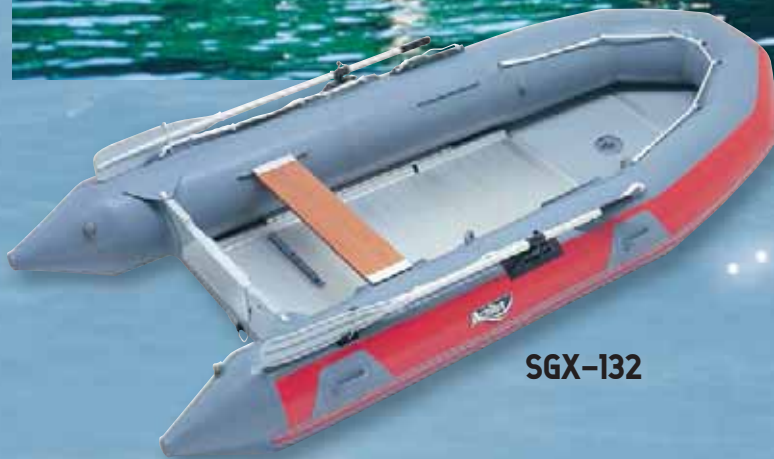
Aluminum Floor and Fiberglass Encased Transom
