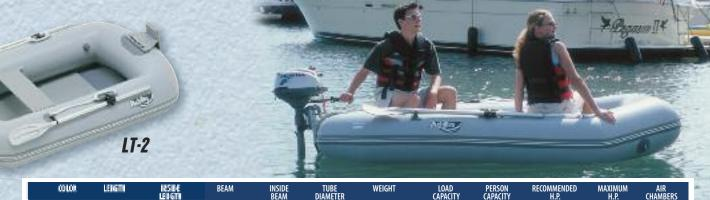
4'1"(124 cm) 1'11" (58 cm) 13"(33 cm) **LT-2** Lt. Gray 7'3" (220 cm) 5' (153 cm) 37 lbs (16.5 kg) 640 lbs (290 kg) 4'8" (142 cm) 2'2" (66 cm) 15" (38 cm) 57 lbs (26 kg) 970 lbs (440 kg) LT STANDARD FEATURES INCLUDE: Achilles CSM reinforced fabric; four-layer seam construction; wood/ Achilles CSM roll-up floor (LT4); hinged wood floor (LT2); full-length rubbing strake; fold-down locking
