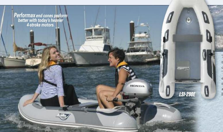
The result is not only a more stylish tender, but also one that outperforms other air floor models by a wide margin. The combination of Performax tubes engineered to work efficiently with today's heavier 4-stroke motors, air keel, and a stiffer air floor result in a smoother handling and better performing boat.
