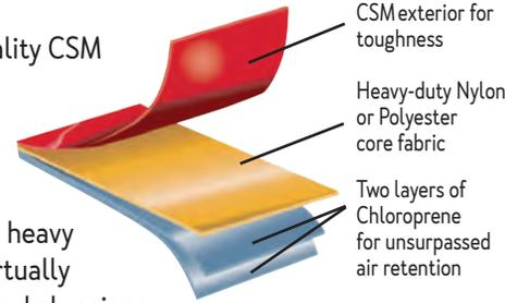
**Designed and built with safety and performance in mind.** From built-in safety features like the strongest four-layer seam construction in the industry to custom designs engineered to complement and enhance the performance of each of our boats, boaters get more out of an Achilles. Our boats are built to not only last, but to also deliver the practicality you expect from an inflatable without sacrificing the performance you want from any boat.
