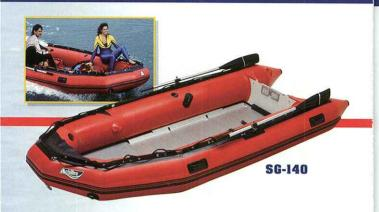
hese "top-of-the-line" models continue to set the standard for inflatable sport boats. Built for high performance with deep "V" trigon air keel hulls, Achilles SG boats offer a roomy, square bow configuration which provides room for extra gear, and an aluminum floor system delivers superior traction, rigidity and durability. Achilles SG sport boats bring performance and practicality together for better water skiing, diving, fishing or all-around sport boating pleasure!
