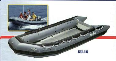
Boats are built tough to work hard for rugged private and commercial use. They are made with an additional heavy-duty layer of 840-denier nylon fabric in a two-ply technique which results in a core fabric even stronger than a single base fabric of equal thickness. A number of exclusive features are built into these boats which combine to bring the advantages of an inflatable together with the demands of tough commercial marine use.
